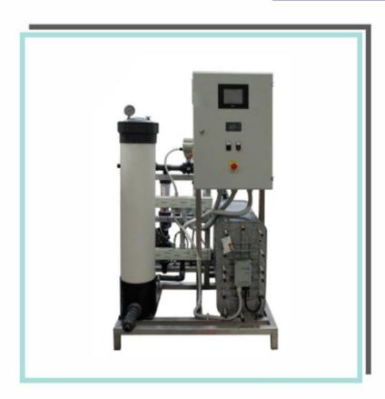
Electrodeionization (EDI) is a technology in which anionic and cationic ions in water are removed from the water by the integrated operation of ion exchange resins and electrical energy to obtain ultra-pure water.
